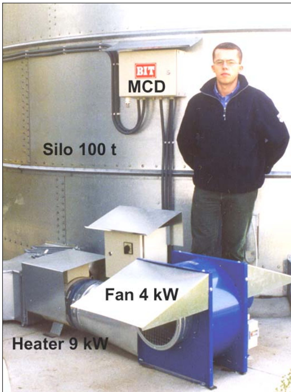
Figure 4.5. Set of equipment for the near-ambient drying of grain - example (courtesy the 'Grzeškowiak' company, Poland).
