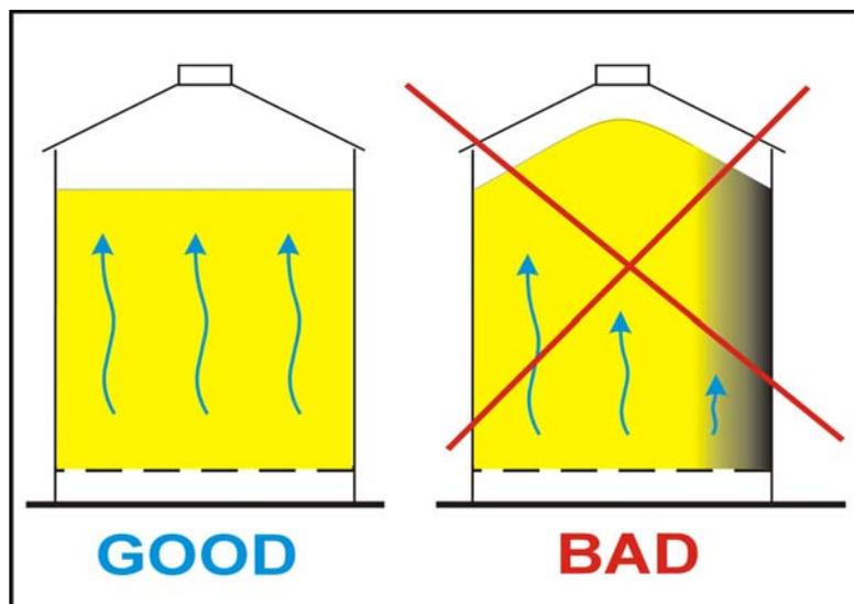
**Figure 3.6.** An even distribution of flow of air on the whole area of the bulk has to be enabled: 1) crop has to have even density in whole space of a silo (crop should be evenly spread throughout the bin) and 2) the grain depth has to be leveled in a silo.
