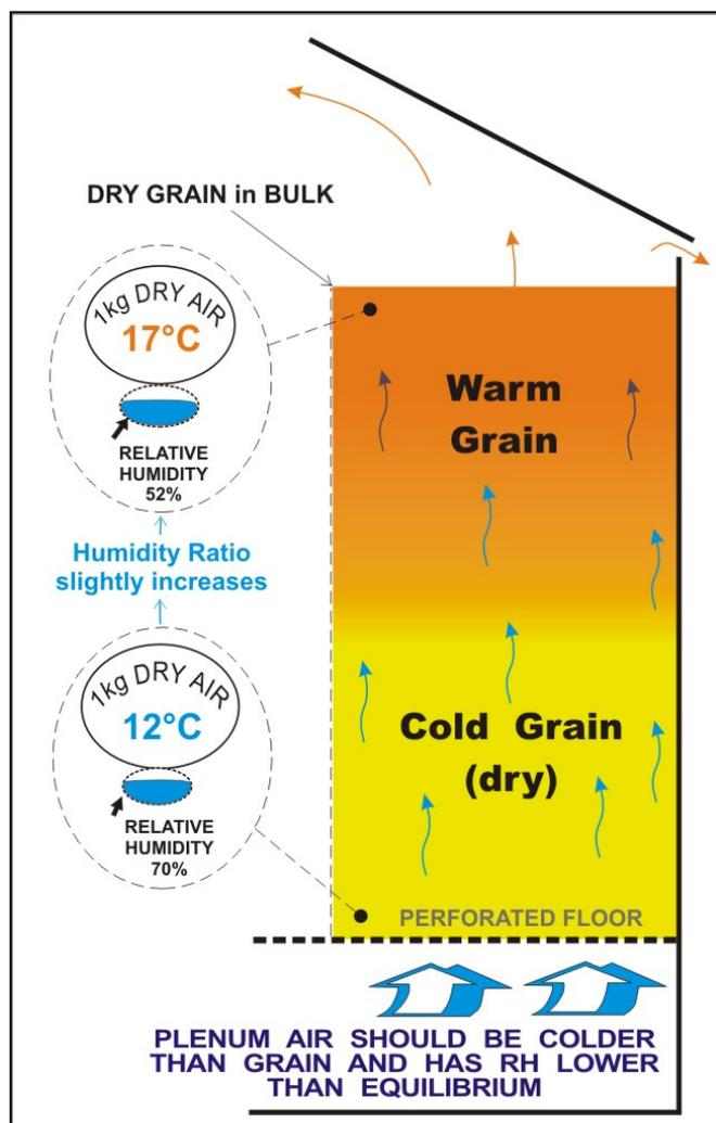
**Figure 3.2.** Changes of air temperature and relative humidity during cooling. Air flows through a deep bed of barley of moisture content 14% w.b. The zone of cold grain moves slowly in the same direction as the flow of the air. The presented values, although they are typical, are only examples. Humidity Ratio in this example increased only 0.1 (g water vapor / 1 kg dry air).
