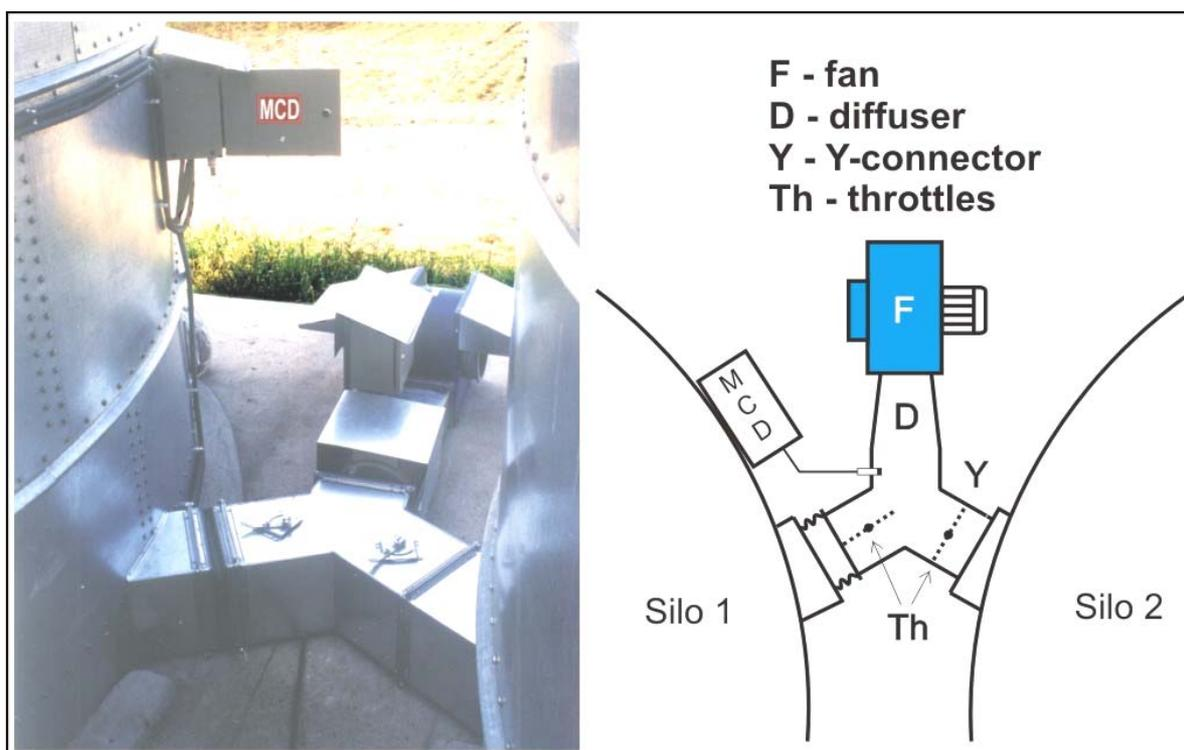
**Figure 3.5.** Example of connection of one fan with two silos using a Y-connector and throttles. This can provide the proper airflow rate for drying grain in one of the silos or the proper airflow rate for cooling grain in both silos simultaneously; “MCD” means Measuring-Control Device.
