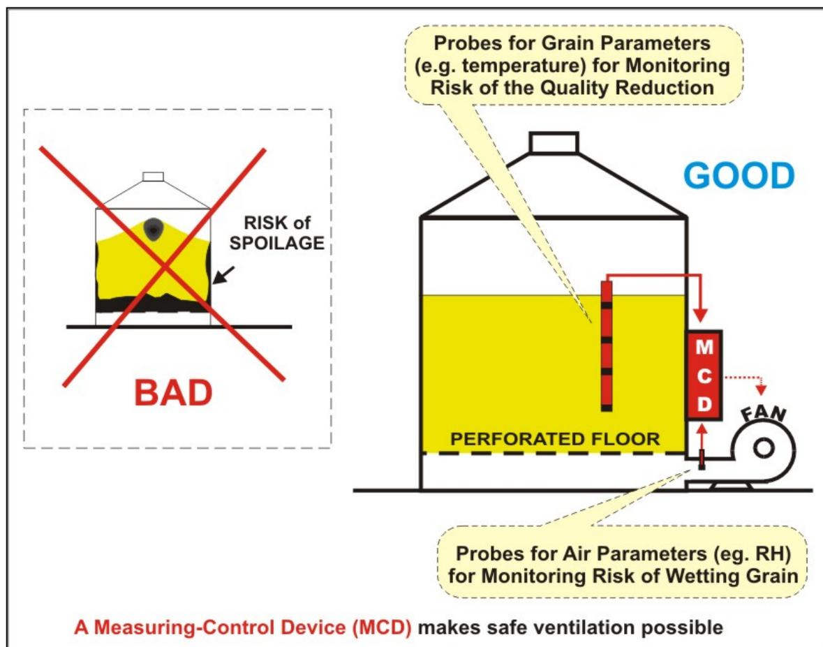
**Figure 3.3.** The set of devices enables the preservation of dry grain with a near-ambient method.
