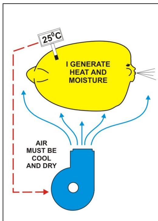
**Figure 3.1. Ventilation of the grain ecosystem.** During the first days after harvest, respiration takes place and grain together with fungi generate heat and moisture, so each kernel in a bulk of grain should have contact with a flow of air that can cool it down and take out this heat and moisture.
